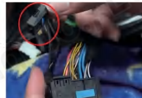
2. Unplug the original fibre optic cable
