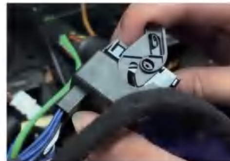
3. Plug the original fibre optic cable into the adapter of our power cable
