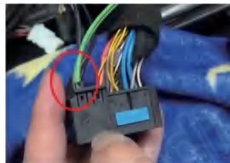
1. OEM fibre optic cable
